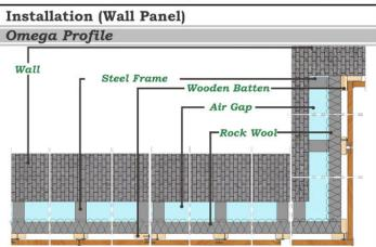
Omega profile can be used to install panels on the wall. Five different options are available. It is also possible to use this system in the installation of ceiling panels.
