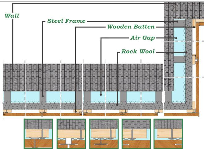
The Omega profile is suitable for mounting wall panels and is offered in five different profile variants. This system can also be utilized for ceiling panel installations.
